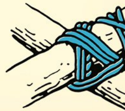
6. Finish your frapping and your lashing with a clove hitch.
