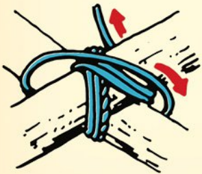
4. Complete three wraps and then prepare for your first frapping.
